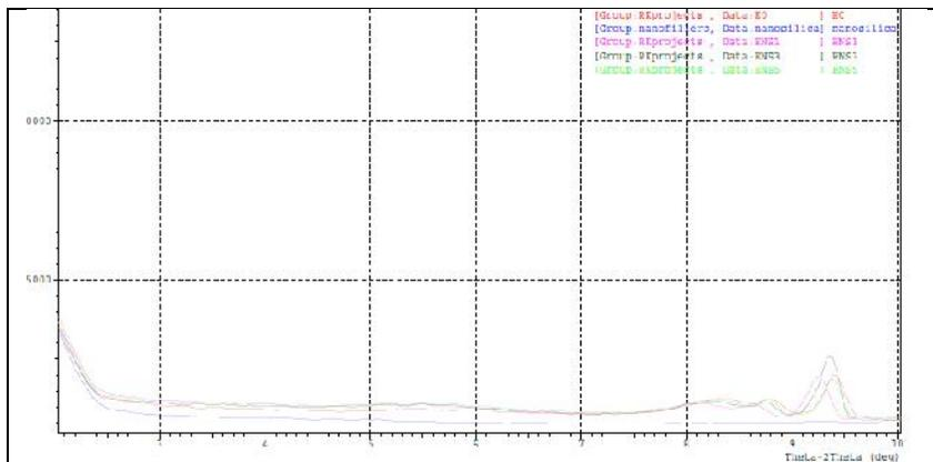
Figure 2: XRD graphs of PNCs with different loading of nano silica
