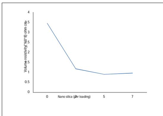
Figure 3: Electrical properties of EPDM Based Nano silica composites
