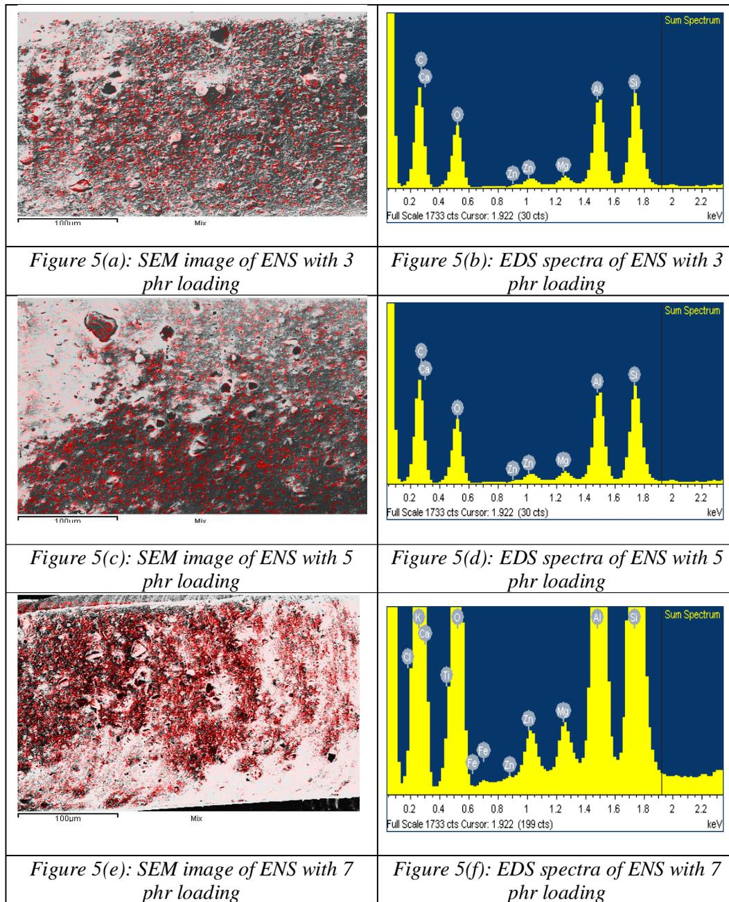
*Figure 5: SEM-EDS Analysis of Nano Silica Mapping in EPDM Rubber*
