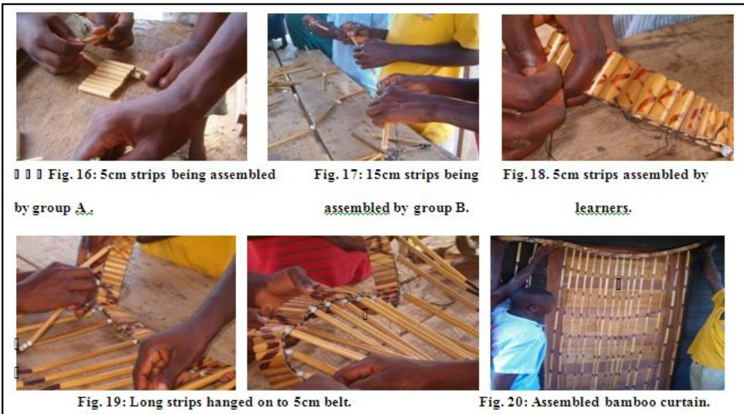
Figures 16 to 20 show learners assembling strips of bamboo into bamboo curtain
