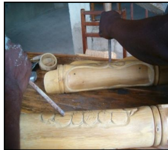
Figure 13: Transferred motifs in groove carving
