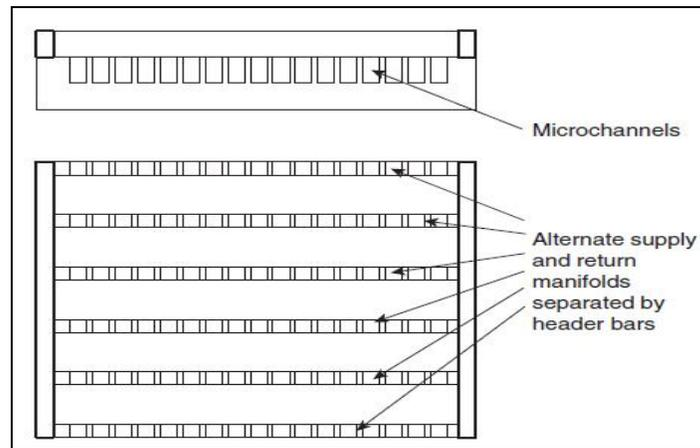
Figure 1: Schematic of Direct Liquid Cooling of a Multichip Module
