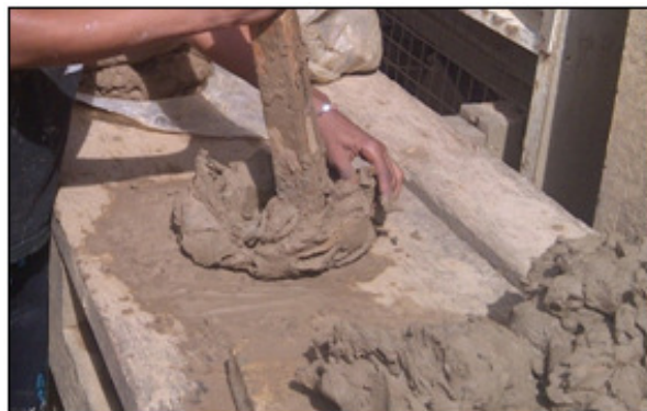
Figure 14: Pounding of lump of clay.
