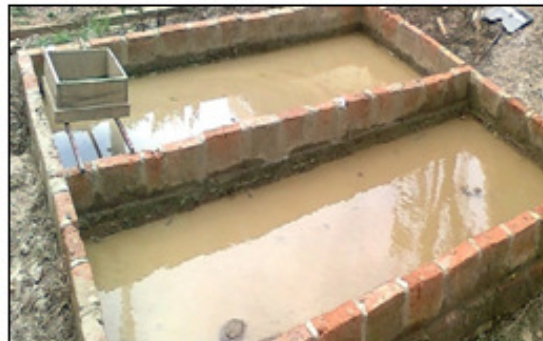
Figure 13: Sieving of clay slip.
