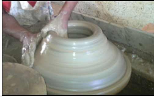
Figure 18: Opening of the clay.
