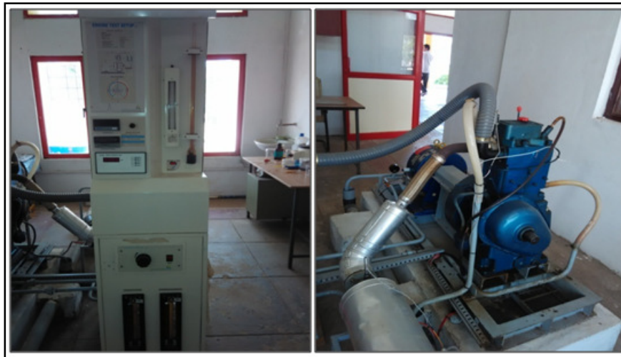
Figure 4: Four Stroke single cylinder VCR diesel engine
