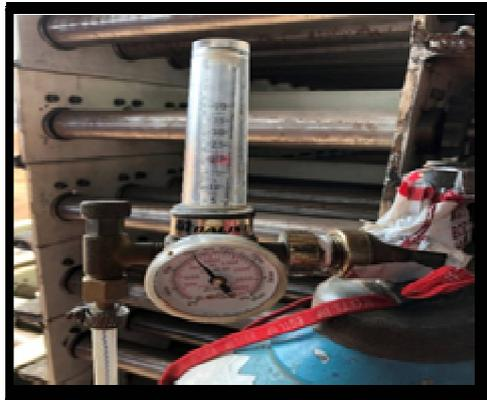
*Figure 3: Shielding Gas Cylinder and Regulator*
