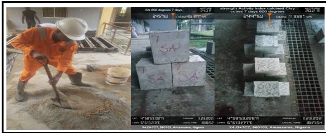
Figure 4: Mixing and Production of Cube Specimens
