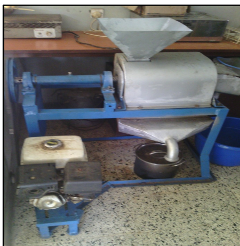
Figure 2: Motorized Cashew apple Juice Extractor
