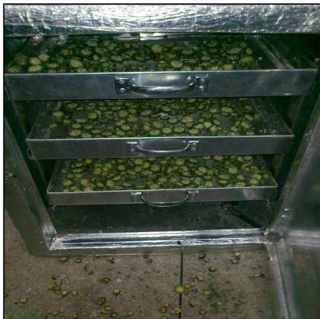
Figure 2c: view of Okra in the cabinet dryer
