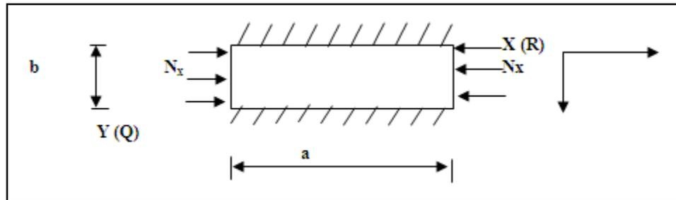
Figure 2: Schematic diagram of axially loaded CSCS Rectangular Plate.
