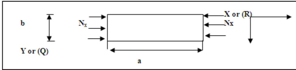
Figure 1: Schematic diagram of axially loaded SSSS Rectangular Plate.
