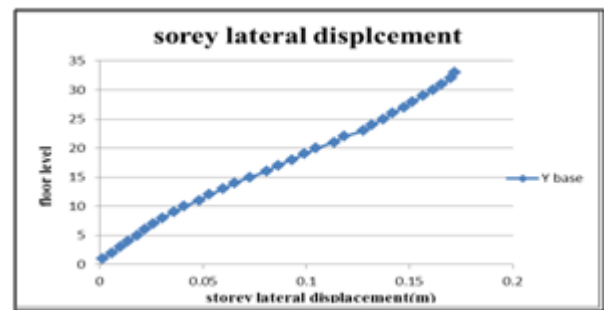
Figure 10: Storey Lateral Displacement for Shear Wall
