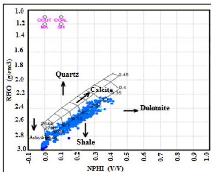
Figure 1: Neutron-Density cross plot to determine the porosity and lithology
