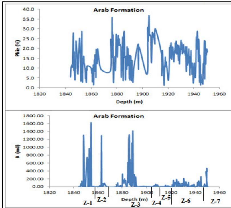
Figure 9: Porosity and permeability variations to depth in Arab Formation
