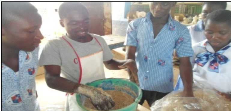
Figure 16 - Preparing the mixture by adding sawdust to glue
