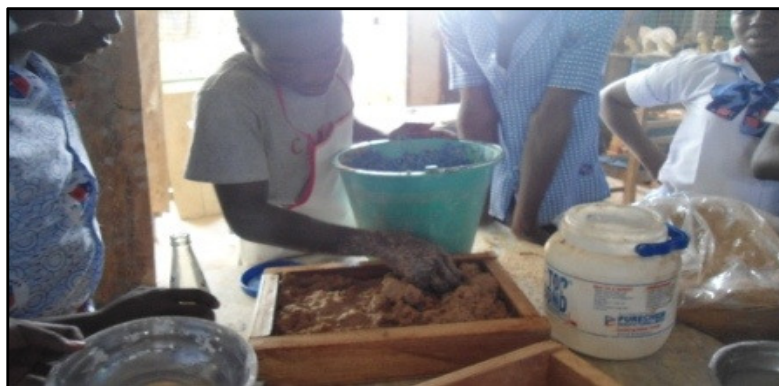
Figure 18 - Prepared mixture was packed into well lubricated moulds
