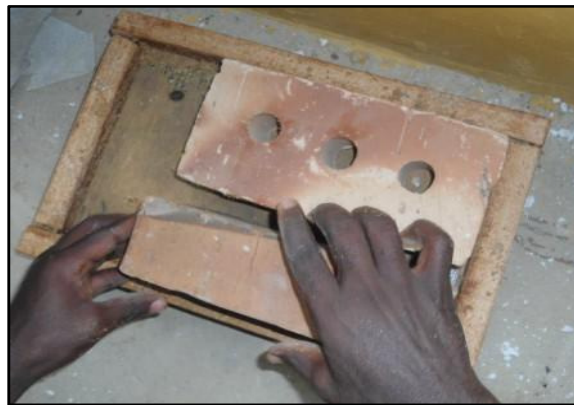
Figure 20 - Bricks were packed on the moulds to exert weight to achieve compactness
