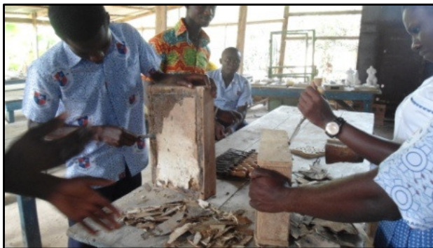
Figure 25 - Using chisels to remove the casts from the moulds
