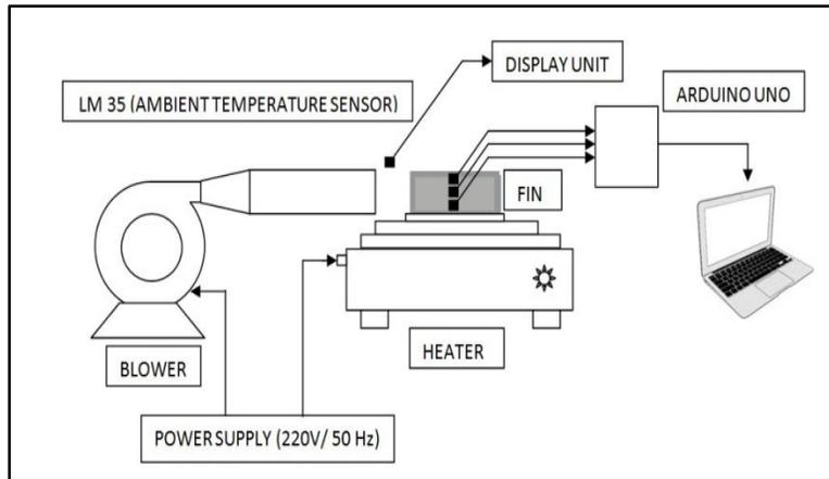
Figure 1: Block diagram of experimental setup
