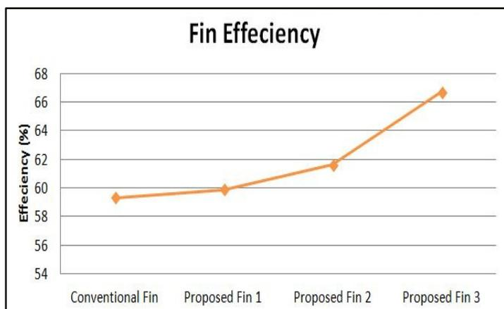
Figure 7: Fin efficiency along with various fins
