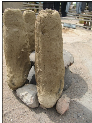
Figure 12: Drying completed moulds
