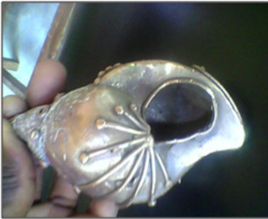
Figure 3: CPSC 4 after casting (No pinholes)
