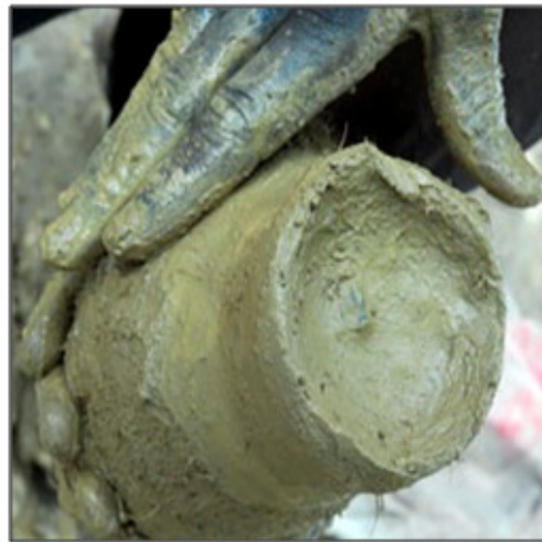
Figure 10: Mould with palm fibre coating
