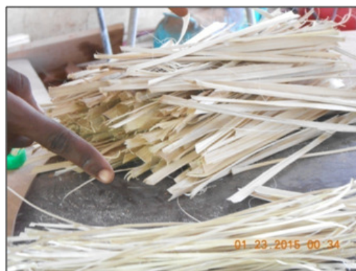
Figure 3: The Bamboo slivers
