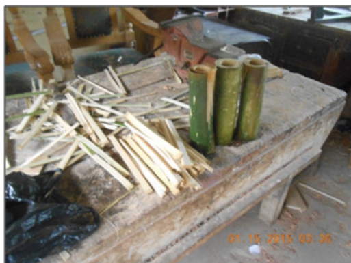
Figure 1: Internodes of Bambusa Vulgaris and splits
