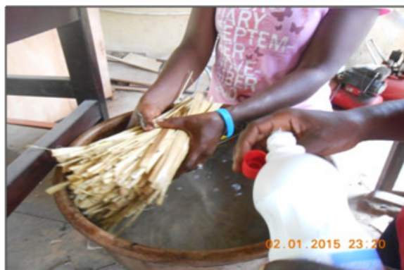
Figure 4: Bleaching of the slivers
