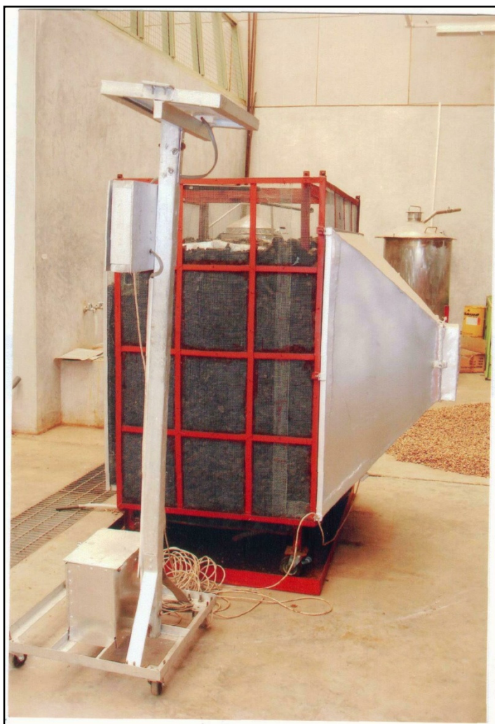
Figure 1: The prototype solar-charcoal cooler developed for laboratory studies
