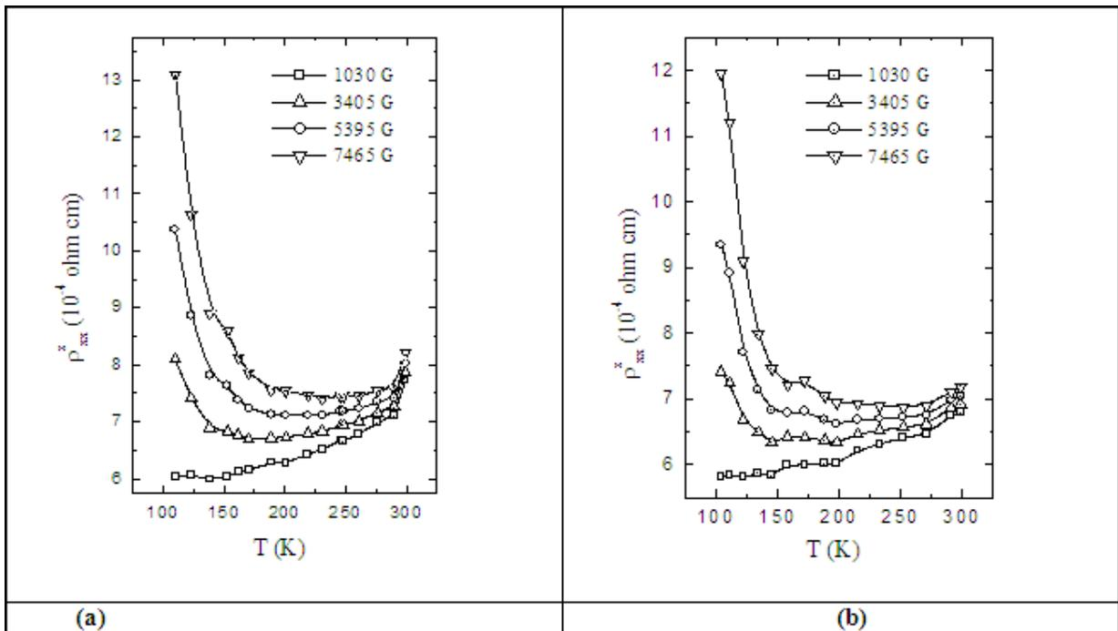
Figure 2: Temperature dependence of the magnetoresistivity: (a) 0.02 at% indium (b) 0.15 at% indium doped bismuth. Applied magnetic field strengths are indicated in the figure.
