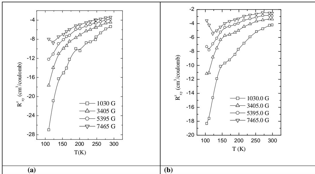
Figure 3: Temperature dependence of the Hall coefficient: (a) 0.02 at% indium (b) 0.15 at% indium doped bismuth. Applied magnetic field strengths are indicated in the figure.
