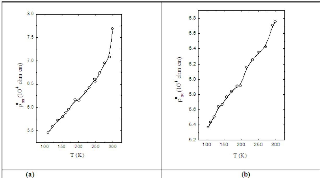
Figure 1: Temperature dependence of the resistivity in the absence of magnetic field: (a) 0.02 at% indium and (b) 0.15 at% indium doped bismuth
