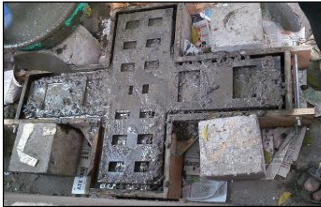
Figure 12: Casting of Test Specimen
