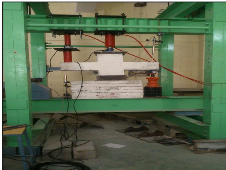
Figure 16: Testing of beam column joint
