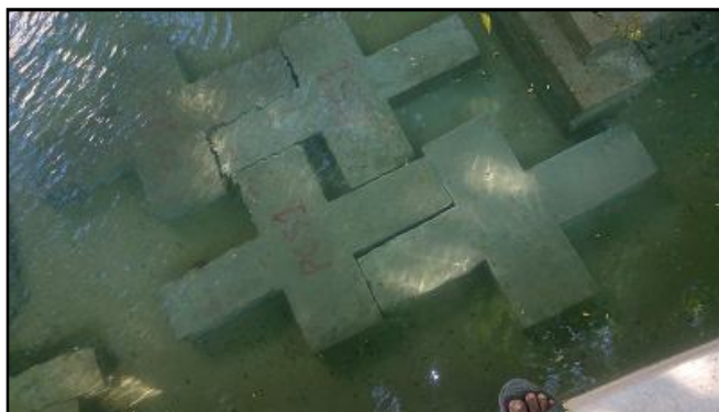
Figure 14: Curing of Specimens
