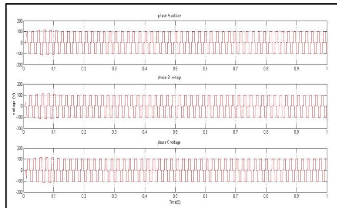
Figure 20: Three Phase Output Voltage wind speed = 10 m/s
