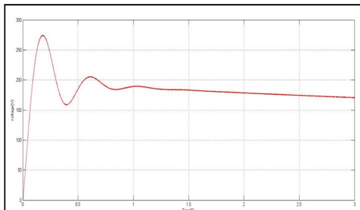
Figure 10: Generator DC Output Voltage @ wind speed = 10 m/s
