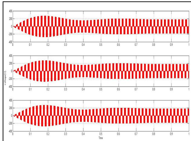
Figure 9: Three Phase Output Voltage wind speed = 7 m/s
