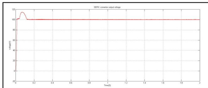
Figure 16: SEPIC CONVERTER Output Voltage @ wind speed = 7 m/s
