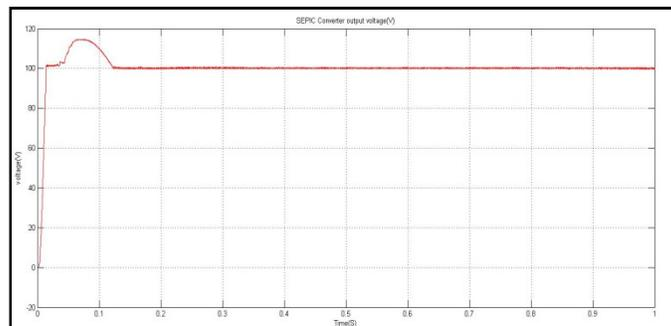
Figure 19: SEPIC CONVERTER Output voltage
