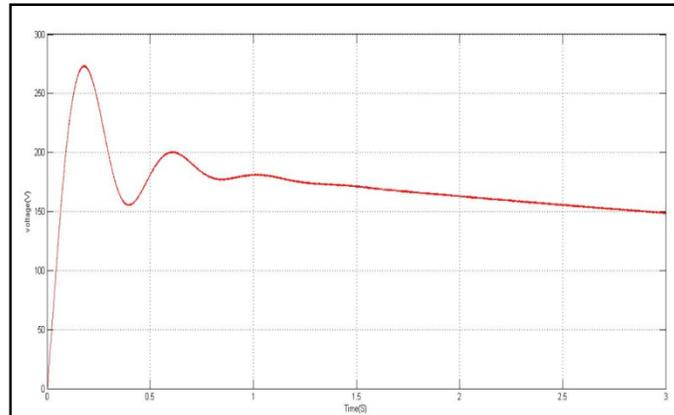
Figure 8: Generator DC Output Voltage @ wind speed = 7 m/s
