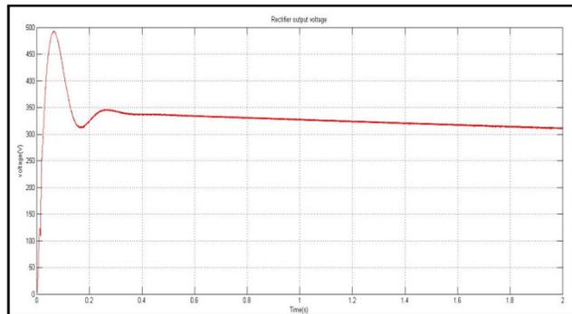
Figure 15: Generator DC Output Voltage @ wind speed = 7 m/s
