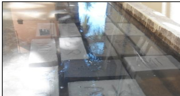
Figure 5: Curing Charcoal Bricks and wood ash bricks in tank with water
