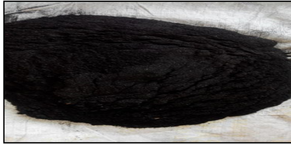
Figure 1: Biochar with pyrolysis of biomass
