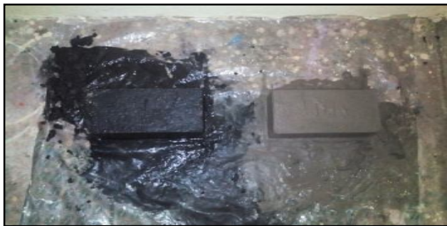
Figure 4: Removal of Charcoal Bricks and wood ash bricks in mould
