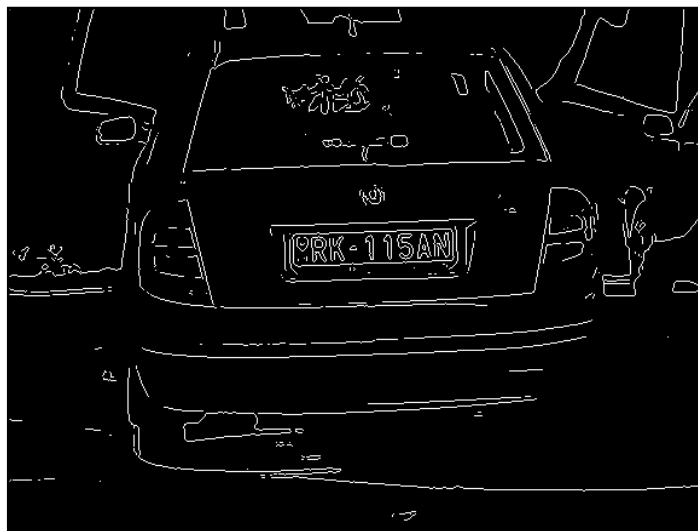
Figure 6: Image after sobel edge detection
