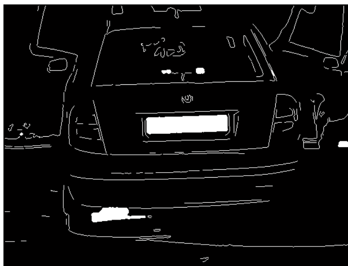
Figure 7: Image after applying sobel edge detection.
