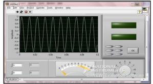
Figure 6: Front Panel of labVIEW software
