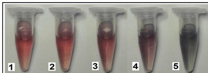
Figure 2: Schematic showing colorimetric detection of melamine in solution using modified gold nanoparticles (AuNPs). (1) AuNP solution without any addition; (2) with the addition of the extract from blank raw milk; (3), (4) and (5) with the addition of the extract containing 1 ppm (final concentration: 8 ppb) melamine, 2.5 ppm (final concentration: 20 ppb) melamine and 5 ppm (final concentration: 40 ppb) melamine, respectively (Adapted from: Ai *et al.*, 2009)
