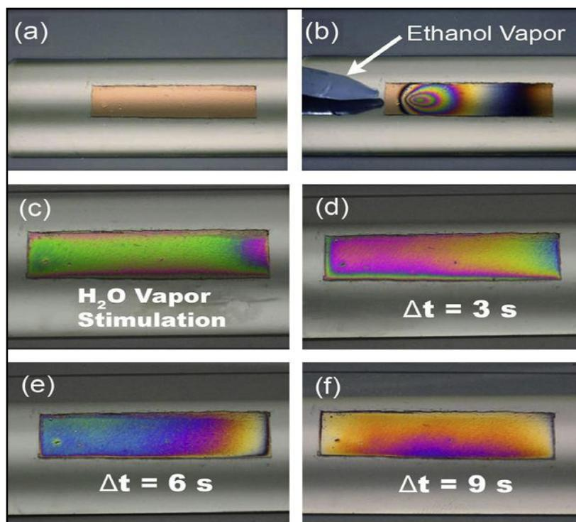
Figure 4: Moisture sensor which utilizes carbon-coated copper nanoparticles dispersed in a polymer matrix (a). Ethanol vapor exposure results in rapid and reversible iridescent coloration (b). Water vapor exposure swells the polymer, which causes the nanoparticles to exhibit larger interparticle separation distances and thus different observable optical behavior (c). As moisture dissipates (d–f), the sensor reverts back to its native state and appearance (Adapted from: Luechinger *et al.*, 2007)
