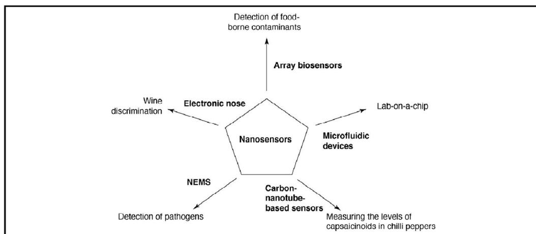
Figure 1: Types of nanosensors and examples of their application in the food sector (Adapted from Sozer *et al.*, 2008)
