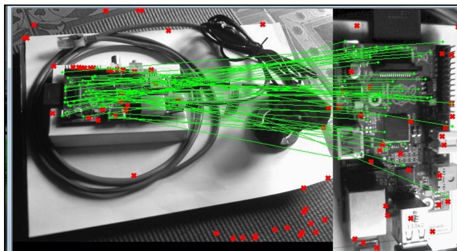
Figure 7: Features matching between object in data base and object in front of the camera
