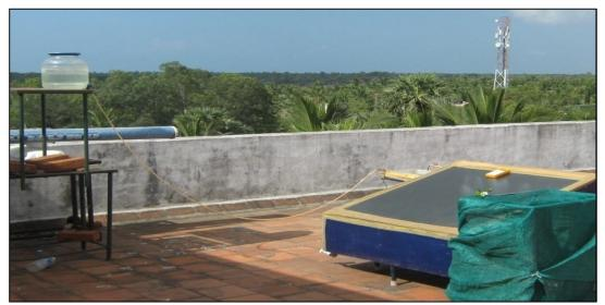
Figure 1: Integrated solar still with green chamber
