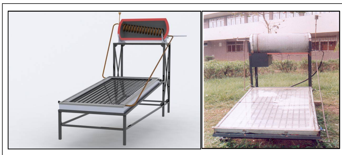
Figure 3: Schematic of SWHS studied with the coiled heat exchanger.
