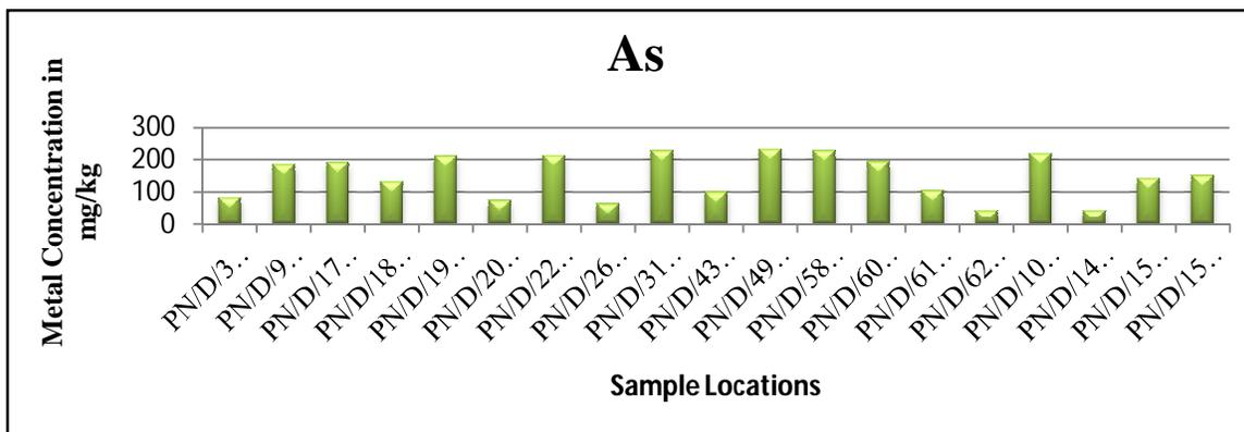
Figure 7: Concentration of Arsenic in Mine Dumps from Enyigba and Environs
