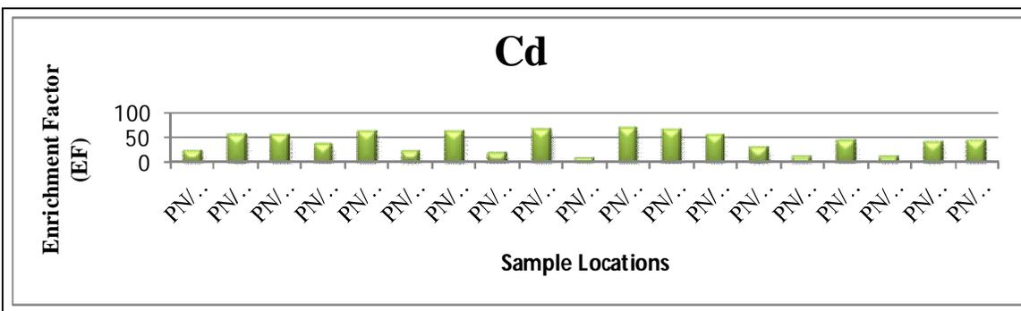
Figure 11: Enrichment Factor of Cadmium in Mine Dumps from Enyigba and Environs.
