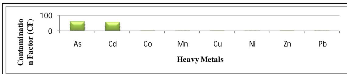
Figure 14: Contamination Factors of Heavy Metals in Mine Dumps from Enyigba and Environs.
