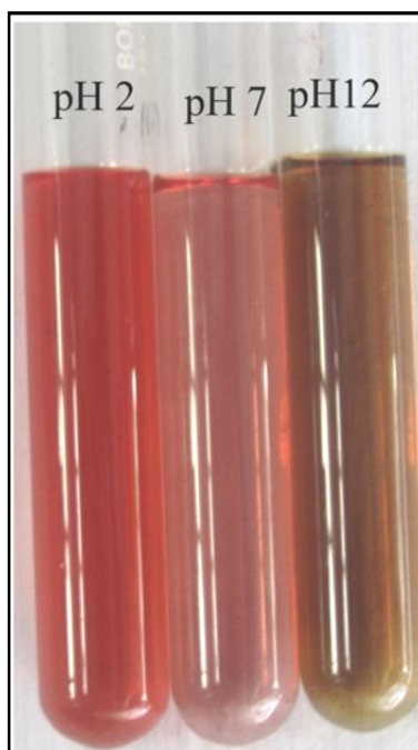
Figure 7: Utility of anthocyanin from Dioscorea as pH indicator
