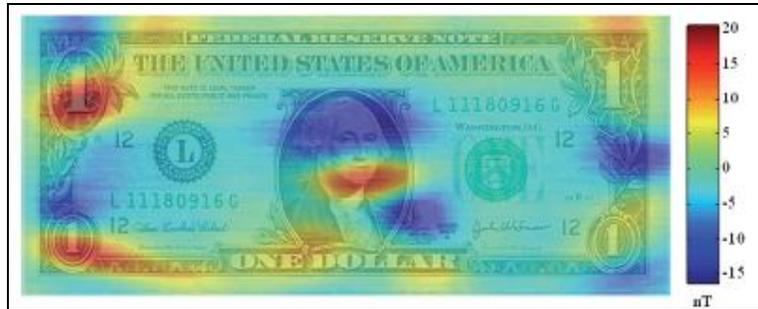
Figure 12: Mapped Gradient Field Of A 1-USD Banknote, As Measured 5 Mm Above The Plane
