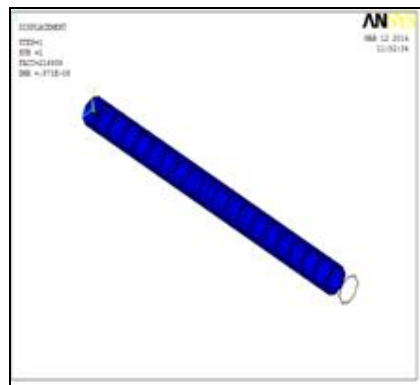
Figure 11: Buckling analysis of steel shaft
