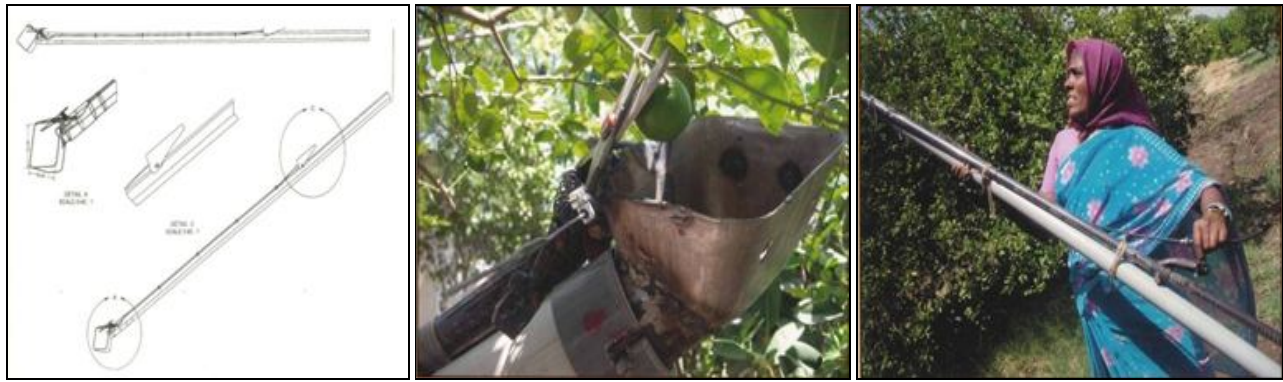
Figure 1: Auto CAD design of manual citrus fruit harvester Plate 1: Cutting mechanism of manual citrus fruit harvester Plate 2: Manual citrus fruit harvester in operation
