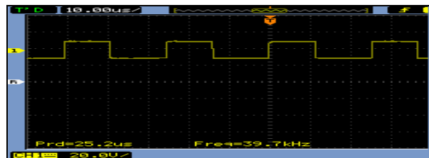
Fig. 29: Gate pulse for MOSFET Switch S 1
