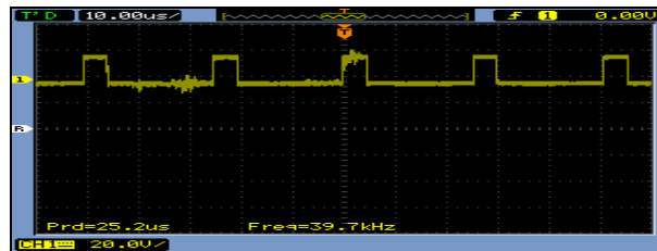
Fig. 28: Gate pulse for MOSFET Switch S
