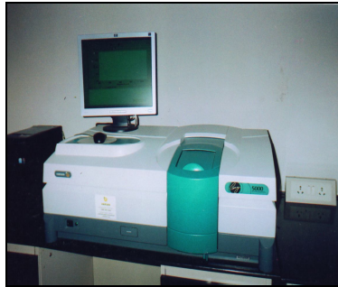
Figure 1: Photograph of Spectrophotometer (Varian Cary 5000)
