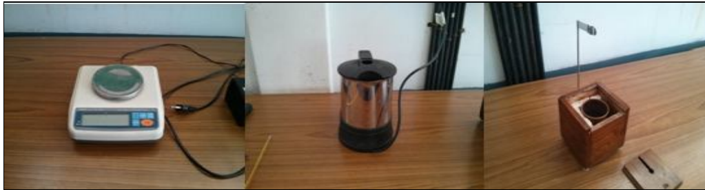
Figure 3: Experimental setup used to determine specific heat
