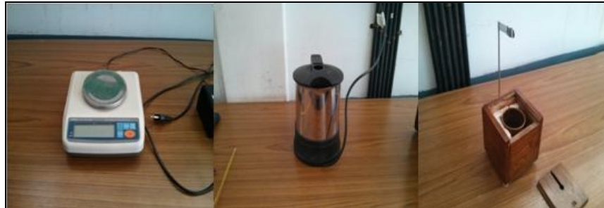
Figure 2.3: Experimental setup used to determine specific heat
