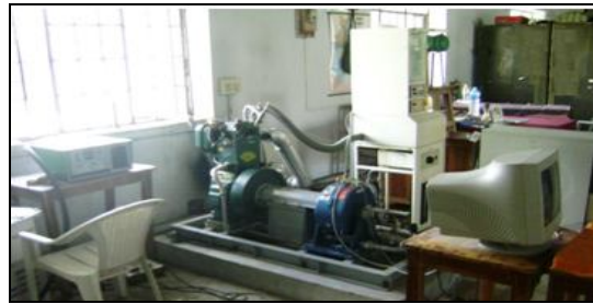
Figure 7: Engine with dynamometer arrangement
