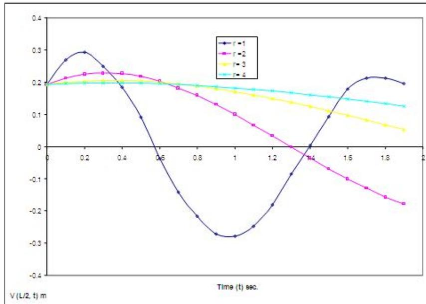
Fig 4: Deflection profile of clamped-clamped uniform Rayleigh beams under the action of moving force for various values of rotatory inertia and fixed value of foundation modulus  $k=20000$  and fixed value of axial force  $N=40000$
