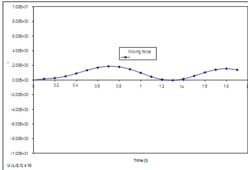
Fig 1: Moving force against Time (t) of the clamped-clamped uniform Rayleigh Beam for fixed values of axial force N and foundation moduli K
