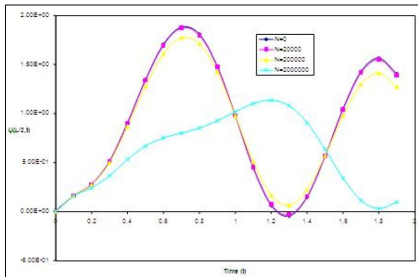
Fig 2: Dynamic response of clamped-clamped uniform beam for various values of axial force N and fixed value of foundation moduli K=40000
