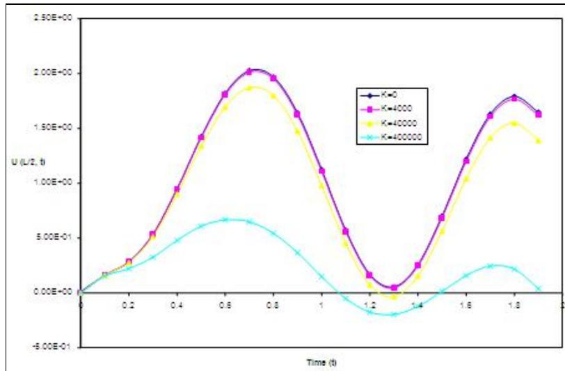
Fig 3: Deflection profile of clamped-clamped uniform beams for various values of foundation moduli  $K$  and for fixed value of axial force  $N=20000$
