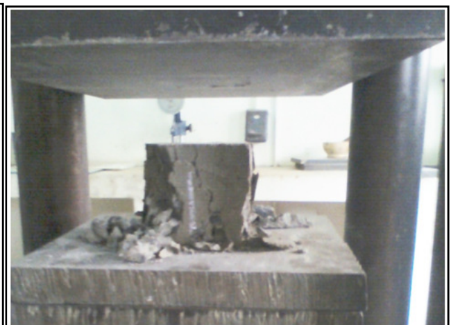
Figure 8: Concrete Cube Immediately After Failure
