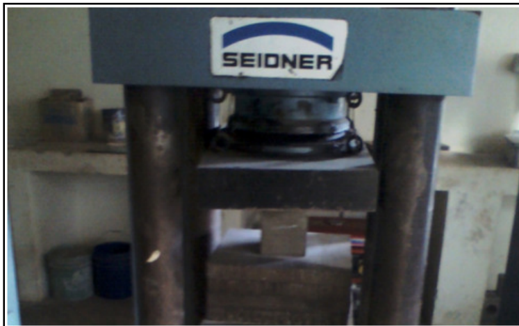
Figure 7: Concrete Cube Loading
