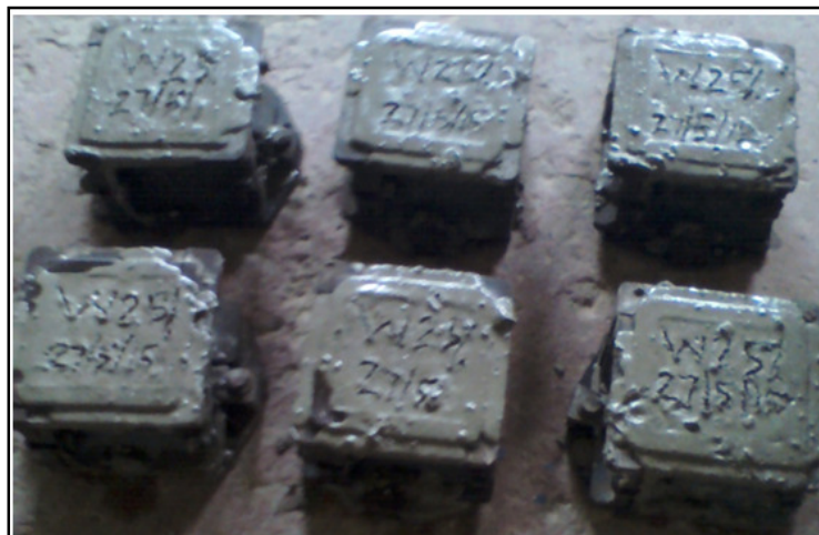
Figure 6: Fresh Cast, Vibrated Concrete Cubes
