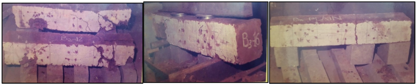
Figure 4a: Showing the failure of reinforced Beam 10mm & Beam 12mm.
