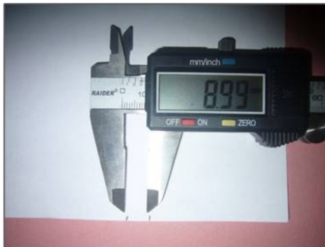
Figure 2: A photograph of an A4 paper, a digital caliper showing how the landmarks were marked (from the radiograph) and measured with the caliper
