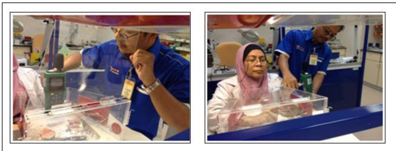
Figure 2: Photos show the procedures of the Indoor Air Quality (IAQ) measurement using the Direct Sense IAQ GrayWolf and DustTrack TSI, USA equipment during the denture trimming process using the X-Dent Box.
