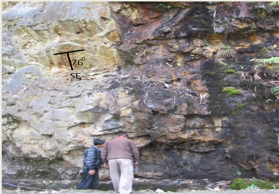
Figure: 3 Shear zone featuring mineralization. Note that schistosity ( S_2 ) strikes N-S to NE-SW dipping SE. (Location near 53 km post)
