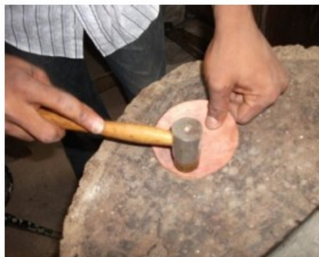
Plate 1 : Sinking a metal disc on a block of wood
