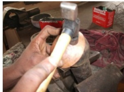
Plate 2 : Raising the disc on a metallic stake
