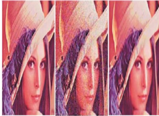
Figure3: Parts Of The Noise-Free, Noisy ( \Sigma=25 , PSNR=20.17db) And The Denoised (PSNR=30.73db) Image.
