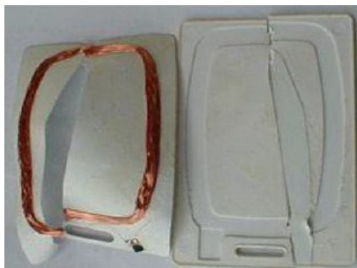
Figure 1: Anatomy of a proximity card: coil and IC
