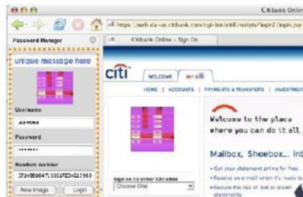
Figure 9: Early mockup displays a visual hash that can be matched to the remote website
