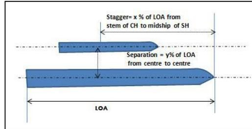
Figure 3: Stagger and separation definition
