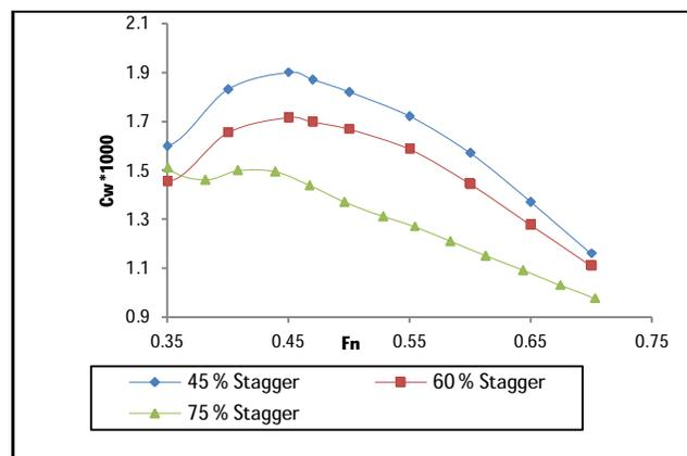
Figure 4:  $C_w$  vs  $F_n$  (Separation = 8.3 %)
