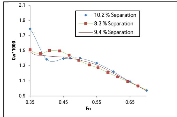
Figure 5:  $C_w$  vs  $F_n$  (Stagger = 75 %)
