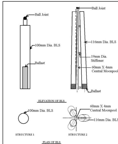
Figure 1: Plan and elevation of scaled model of BLS
