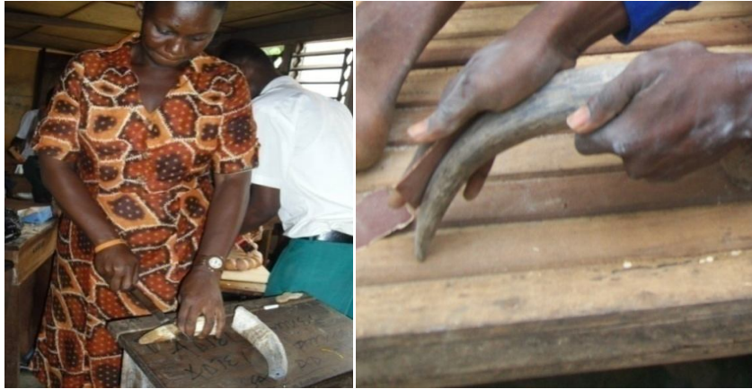
Figure 4c: cutting the cow horns Figure 4d : sanding the cow horns
