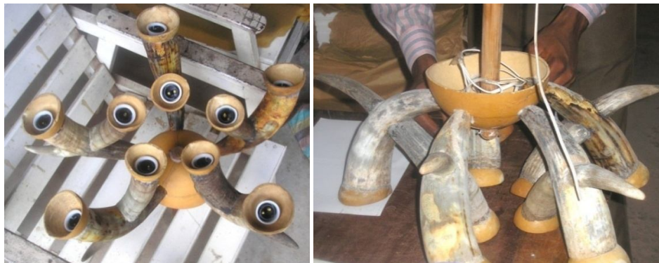
Figure 4g: fixing the lamp holders Figure 4h :fixing the bamboo holder and wiring
